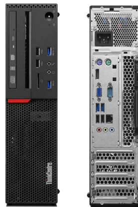
ThinkCentre M700 SFF front and back view (with optional card reader and front USB 2.0)
